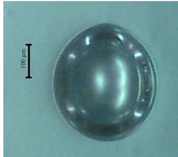
**Fig. 4** Optical image of a laser-induced cavitation bubble. The laser beam was delivered from the bottom and the ultrasound transducer was positioned at the top, as indicated in Fig. 1.
