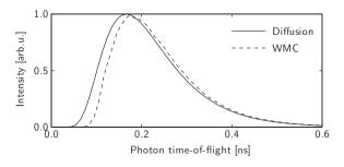
**Fig. 6** Illustration of the breakdown of the diffusion approximation in the low albedo regime of photon migration. In this particular case, the data correspond to an infinite (interstitial) geometry using a 15-mm source-detector separation, with  $\mu'_{s}$ =7.5 cm<sup>-1</sup>, and  $\mu_{a}$ =0.5 cm<sup>-1</sup>.
