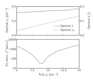
Fig. 4 WMC fitting procedure of the experimental data featuring the 2-ml added ink absorption series measurement at 660 nm,  $\rho$  = 14.7 mm.
