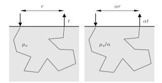
**Fig. 1** In WMC, the shapes of the photon paths are determined only by the phase scattering function and the sequence of random numbers. Paths generated by simulations in nonabsorbing media can hence be linearly scaled to apply for different values of  $\mu_s$ . The illustration is adapted from Ref. 12.
