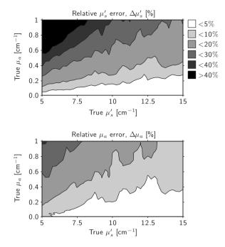
**Fig. 8** Relative errors due to diffusion modeling when fitting is performed between the 80% level (of peak maximum) on the rising flank and the 1% level on the tail. As in Fig. 7, diffusion modeling results in overestimation of both scattering and absorption. The gray scale applies to both graphs.
