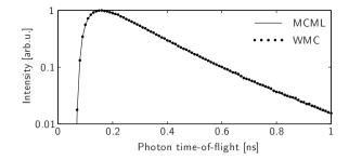
**Fig. 5** Illustration of the agreement between MCML and the proposed WMC. In this particular case, the source-detector separation is 15 mm,  $\mu'_s$ =5 cm<sup>-1</sup>, and  $\mu_a$ =0.1 cm<sup>-1</sup>.
