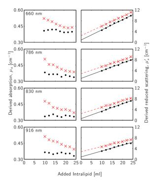
**Fig. 12** The results from the added scatterer series (adding further Intralipid to a liquid phantom based on ink and Intralipid). Derived optical properties are given both for diffusion-based evaluation (crosses) and WMC-based evaluation (circles). The results are to be compared with the simulation results presented in Fig. 10.
