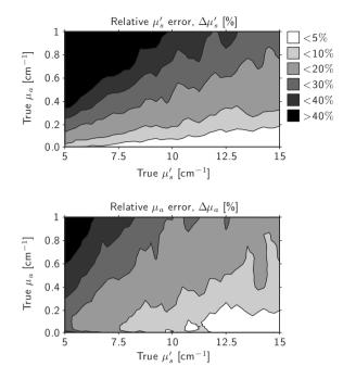
**Fig. 7** Relative errors due to diffusion modeling. Since the relative errors are positive throughout the examined range, diffusion modeling results in overestimation of both scattering and absorption. Fitting is performed between the 50% level (of peak maximum) on the rising flank and the 20% level on the tail. The gray scale applies to both graphs.
