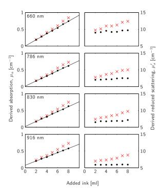
**Fig. 11** The results from the added absorber series (adding ink to a liquid Intralipid phantom). Derived optical properties are given both for diffusion-based evaluation (crosses) and WMC-based evaluation (circles). The results are to be compared with the simulation results presented in Fig. 9.
