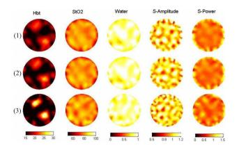
**Fig. 6** Simulation of two-target phantom with known contrast in total hemoglobin (Hbt). Row (1) involves four wavelengths (695, 750, 800, and 830 nm), row (2) involves six wavelengths (695, 710, 750, 780, 800, and 830 nm), and row (3) involves 12 wavelengths (695, 700,710, 725, 735, 750, 770, 780, 800, 810, 820, and 830 nm). These choices match the experimental study shown in Fig. 6.
