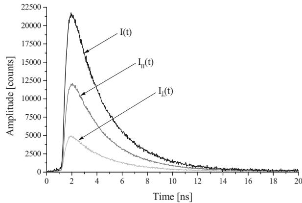
**Fig. 3** Fluorescence intensities  $I_{\parallel}(t)$ ,  $I_{\perp}(t)$ , and  $I(t) = I_{\parallel}(t) + 2I_{\perp}(t)$  of stably transfected T47D-EYFP-Mem breast cancer cells. Excitation wavelength: 470 nm; detection range:  $\lambda \geq 515$  nm.
