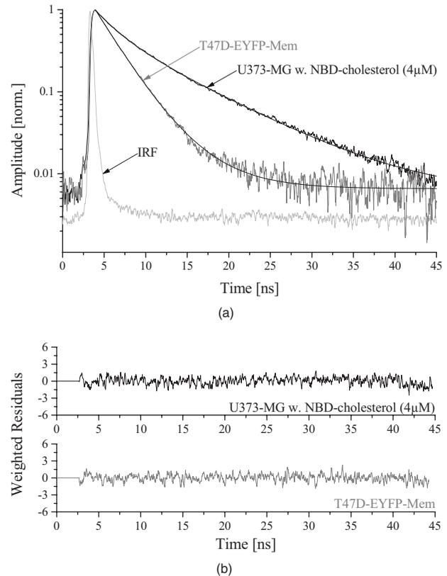
**Fig. 2** Normalized fluorescence intensity  $I(t)$  of U373-MG glioblastoma cells incubated with NBD-cholesterol ( $4 \mu\text{M}$ , 60 min) and of stably transfected T47D-EYFP-Mem breast cancer cells including biexponential fitting curves and IRF (a) with weighted residuals (b). Excitation wavelength: 470 nm; detection range:  $\lambda \geq 515$  nm.
