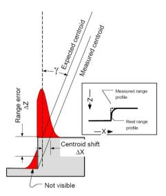
**Fig. 5** A range discontinuity results in a shift ( $\Delta x$ ) in the position of the centroid in a triangulation laser range scanner. This results in a range error  $\Delta z$ . [modified from Fig. 7(a) of Ref. 7].
