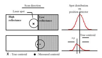
Fig. 7 Transitions between regions of different surface reflectivity can affect the accuracy of the range measurement (Fig. 1 of Ref. 36).
