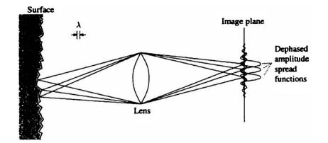
Fig. 3 Speckle noise arises from the interference of a series of diffraction patterns, each generated by a speckle element. (modified from Fig. 2.11 of Ref. 25).
