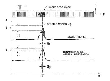
Fig. 4 Speckle noise is reduced by integrating the measurement over several sampling intervals. (modified from Fig. 3 of Ref. 23).
