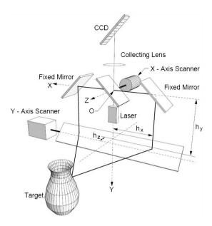
Fig. 1 Example of a fixed-viewpoint laser range scanner employing dual-axis galvanometer-controlled rotating mirrors [modified from Fig. 6(b) of Ref. 10].
