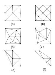
Fig. 12 Facet ratio is most effective for regularly-spaced data, such as (a) and (b). As measurement distribution becomes less regular, facets with large facet ratios can emerge regardless of their relative range measurements.
