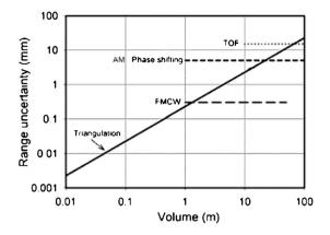
**Fig. 2** Common range uncertainties for Amplitude-Modulation Continuous Wave (AM), Frequency-Modulation Continuous Wave (FMCW), Time-of-Flight (TOF) and triangulation scanners up to 100-m effective range (referred to in this figure as volume). The range measurement uncertainties of all but the triangulation scanners are considered constant with respect to range. [modified from Fig. 2(b) of Ref. 16].
