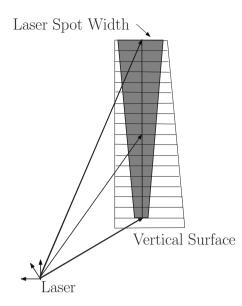
Fig. 9 Assuming the scanner position is limited to within a metre or two of ground level, the lateral measurement uncertainty increases as the height of the structure increases due to the increase in the distance between the scanner and the surface.
