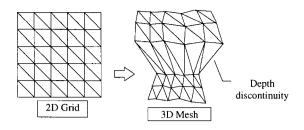
**Fig. 11** Range discontinuities result in elongation of Delaunay facets when viewed in three dimensions (Modified from Fig. 4 of Ref. 38).
