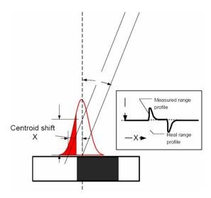
**Fig. 8** Discontinuity in surface reflectivity results in a shift  $(\Delta x)$  in the position of the centroid in a triangulation laser range scanner. This results in a change in return signal intensity. [modified from Fig. 7(b) of Ref. 7].
