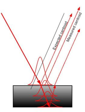
Fig. 6 Range errors can result from the laser penetrating the surface of the material being scanned. (modified from Fig. 6 of Ref. 7).
