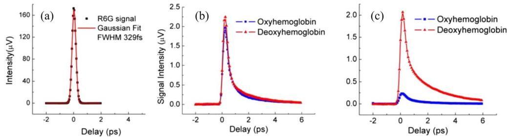
**Fig. 1** (a) TPA signal from R6G with 810-nm pump at 10 mW and 740-nm probe at 6.4 mW. (b) ESA signal from oxyhemoglobin and deoxyhemoglobin with pump wavelength at 810 nm and probe wavelength at 740 nm; pump power was 10 mW and probe power was 6.4 mW. (c) ESA signal from oxyhemoglobin and deoxyhemoglobin with pump wavelength at 740 nm and probe wavelength at 810 nm; pump power was 2.4 mW and probe power was 10 mW.
