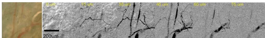
**Fig. 3** Bright-field image and corresponding two-color ESA images at increasing imaging depth (pump at 735 nm with 4-mW power and probe at 810 nm with 1.6-mW power). (Color online only.)
