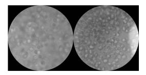
**Fig. 7** Widefield image of cells imaged in reflectance labeled with gold nanoparticles. The image taken with the 4M device (right) shows the significance of the internal lens surface reflections. The bright region on the right of the image is due to a single surface reflection from an AR-coated lens. A similar image taken with a Zeiss Axiovert 100M is shown (left) for comparison. Black circular masks limit the FOV to 250  $\mu$ m for each image.
