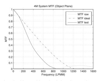
**Fig. 5** Plot of the MTF of the combined relay and 4M optical systems measured by the tilted-edge method. The dashed line represents the ideal MTF. The solid dark curve is the calculated MTF, and the solid light segment (raw data) was assumed to be noise and was blocked by a threshold level. The computed Strehl Ratio was 0.67 for the device with 0.4 NA.
