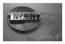
**Fig. 3** Assembled 4M device shown above a United States penny for scale. The system incorporates the micromounted lens, hybrid printed lenses, beamsplitter, illumination optics, and fiber holder. The image is formed at the location where the detector will be integrated in future devices. This intermediate image is relayed by optical bench relay lenses to a CCD camera for testing purposes.
