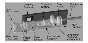
**Fig. 1** Rendered design of the 4M device that illustrates optical components mounted on the MOT substrate. In the future completed device (not shown), the image sensor is to be mounted on a PCB and attached to the 4M device walls.
