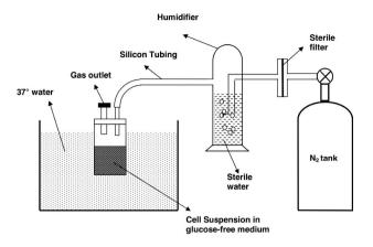
Fig. 1 Setup for the oxygen-glucose deprivation experiments.
