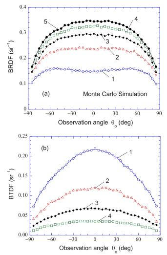
Fig. 8 Monte Carlo simulation of (a) BRDF and (b) BTDF at normal incidence.
