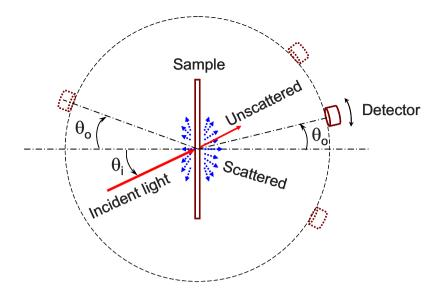
Fig. 1 Schematic of volume scattering by a slab and the laser scatterometer. The unscattered light is the transmitted collimated beam. The observation angle  $\theta_o$  is relative to the surface normal of the sample and defined separately for BRDF and BTDF measurements. In the experiments, the direction of the laser is fixed. The sample can be rotated to change the incidence angle  $\theta_i$  and the detector can be rotated around the sample.
