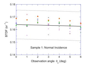
**Fig. 7** BTDF of sample 1 at normal incidence for eight measurements in the observation angle range from 0 to 6 deg. The solid line represents the quadratic fit of the average BTDF, discussed previously in Fig. 3, whereas the dashed lines denote the uncertainty bounds with 95% confidence interval.
