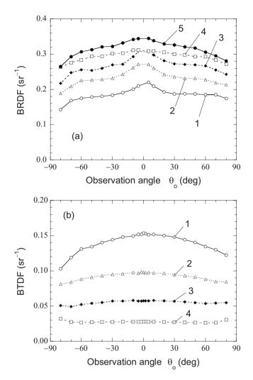
Fig. 2 Measured (a) BRDF and (b) BTDF, averaged over the two polarizations, at normal incidence for  $\lambda$ =635 nm.
