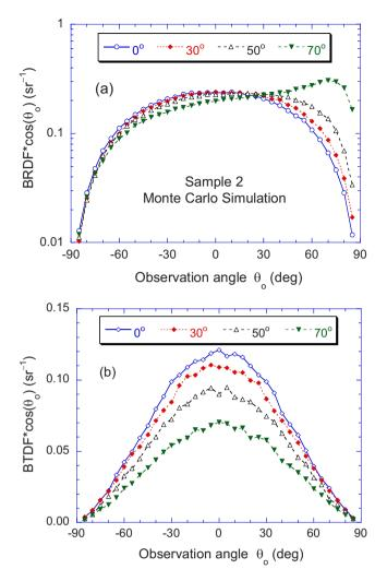
Fig. 9 Monte Carlo simulation of the (a) BRDF and (b) BTDF of sample 2 at different incidence angles.
