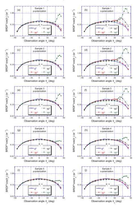
Fig. 4 BRDF of all five samples at various incidence angles for both *p*- and *s*-polarizations.
