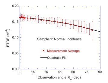
**Fig. 3** Average of eight BTDF measurements for sample 1 and the fitted polynomial curve. The error bars show the measurement uncertainty with 95% confidence interval.
