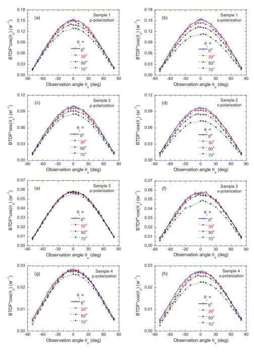
Fig. 5 BTDF of the four thin-film samples at various incidence angles for both polarizations.
