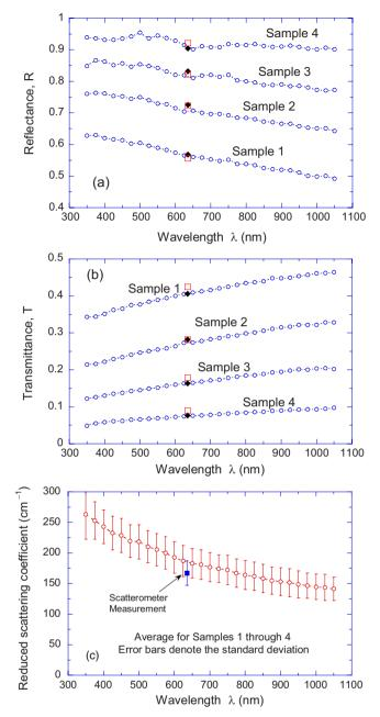
**Fig. 10** Spectral, directional-hemispherical (a) reflectance and (b) transmittance of the thin-film samples measured with an integrating sphere at normal incidence. The square marks represent data integrated from the scatterometer measurements; diamond marks represent data obtained with the diode laser at 635-nm wavelength and the integrating sphere. (c) Reduced scattering coefficient calculated from R/T, as compared with that obtained previously from the scatterometer measurements.
