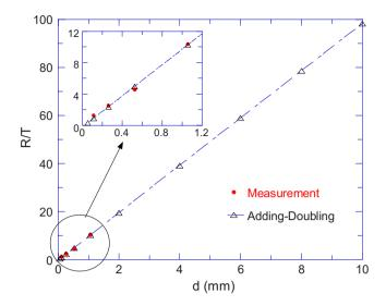
**Fig. 6** The ratio of R/T obtained from the integration of measured BRDF and BTDF (dots) and that calculated using adding-doubling method (triangles), where the inset shows the results for a small *d* range. The parameters used for the calculation are  $\sigma' = 167 \text{ cm}^{-1}$  and g = 0.9.
