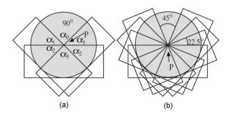
**Fig. 3** Glass plate MDE assembled in the lab, three and seven glass versions. The reference arm light beam represented by the gray area is perpendicular to the paper plane, and it is centered on point P.
