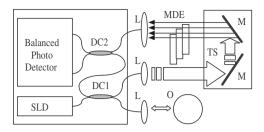
**Fig. 1** Diagram of the multiple delay OCT system. SLD: superluminescent diode; DC1, DC2: single-mode directional couplers; L: lenses; M: mirrors; MDE: multiple delay element with three layers, which introduces four reference paths; TS: translation stage; and O: object to be measured.
