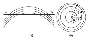
**Fig. 2** (a) B-scan image of a metal sphere obtained when using a three-2 layer MDE. (b) C-scan image corresponding to the A-A' plane from the left image.
