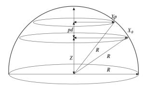
**Fig. 4** Geometrical relations on the calibration sphere, showing the geometrical relationships between R, Z,  $X_p$  and d.
