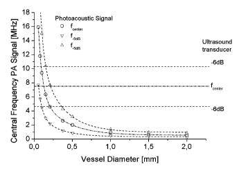
**Fig. 3** Central frequency and –6-dB bandwidth of the photoacoustic signal as a function of vessel diameter. The central frequency and –6-dB bandwidth of the 7.5-MHz transducer are plotted as well (horizontal dashed lines).
