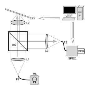
**Fig. 1** Schematic of the raster-scanning scatter imager. The solid semitransparent arrows show the illumination and detection beam paths. Identical achromatic lenses (L1 and L3), the objective lens (L2), the beamsplitter (BS), the illumination fiber (F1), and the detection fiber (F2) are all arranged in the standard confocal geometry. The distal end of the detection fiber is coupled to a CCD-based imaging spectrometer (SPEC), which records the remitted irradiance spectrum.
