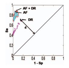
**Fig. 12** ROC plot showing how the optimum classification accuracy couple (Se and Sp) is determined for each spectroscopic modality: blue data cluster, AF; pink, DR; and red, bimodality (DR+AF). The current plot illustrates the determination of the optimum (Se, Sp) couple for the discrimination of N and AH using DR; the data point that is the farthest away at distance *d* is kept as the optimum classification result.
