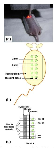
**Fig. 1** (a) An anesthesized mouse on the heated blanket during spectroscopic measurement. The optical fiber probe was put in gentle contact with the skin through a plastic pattern stuck on the mouse's back to localize spectroscopic evaluation spots. (b) Schematic of the plastic pattern dimensions and black ink tattoo used to localize each 6-spot row along the backbone. (c) Schematic showing the method used to localize histological evaluation sites.
