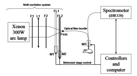
Fig. 2 Schematic diagram of the bimodal spectroscopy system used to acquire mouse skin spectra *in vivo* using a short arc lamp (300-W xenon). F1: anticaloric filter; L1: convex lens; FL1 and FL2: high-pass and low-pass linearly variable filters; Fexc: excitation optical fiber; M1, M2, and M3: motorized micrometric translation stages.
