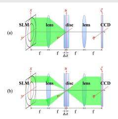
Fig. 1 Transmission model of the collinear algorithm for (a) a writing process and (b) a reading process.
