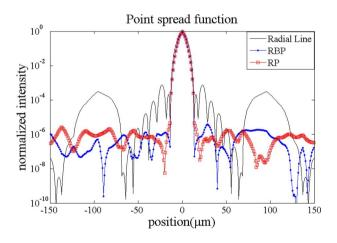
Fig. 3 PSF with different kinds of modulation.
