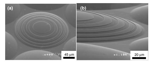
Fig. 2. SEM images. (a) overview and (b) enlarged view of an SiO<sub>2</sub>-based hybrid lens. Reprinted with permission from *Optics Express*. Copyright 2008, Optical Society of America [8].
