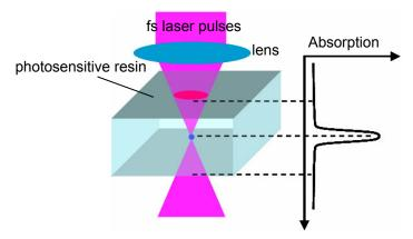
Fig. 1. Schematic illustration of multiphoton absorption induced using femtosecond laser pulses.
