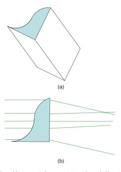
**Fig. 5** The odd-symmetric lens consisting of two half-positive and half-negative cylinders. (a) a perspective view. (b) The effect of that lens is to produce a half-diverging and a half-converging beam. This type of lens could correct the cross-comatic vergence error when aligned along the 45-deg diagonal.
