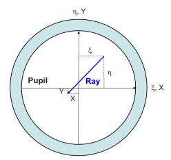
**Fig. 4** Front view (projection on the *XY* plane) of a skew ray similar to that of Fig. 3. There are four possible components of the vergence error because each transverse aberration depends on both pupil coordinates.
