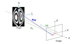
**Fig. 3** Trajectory of a general skew ray from the pupil to the image. Skew rays will never cross the axis so that the scalar  $\Delta z$  and its associated vergence are not well defined.
