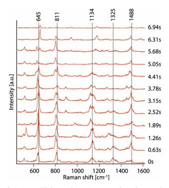
**Fig. 6** Temporal behavior of a SERS spectrum obtained at a single point in a living macrophage cell. The exposure time was 0.5 s, and SERS measurements were taken every 0.63 s.
