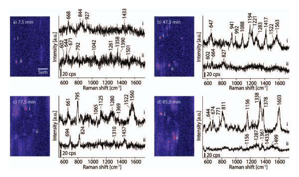
Fig. 5 SERS spectra obtained in selected frames of the time-lapse SERS observation shown in Fig. 4. The bar in the spectra indicates 20 photon counts/s.
