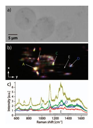
**Fig. 1** (a) Bright-field and (b) a SERS image of macrophage cells with gold nanoparticles. Raman spectra in the spots indicated as A to E are shown in (c). For taking the SERS image, the samples were irradiated with 785-nm continuous-wave laser light of intensity of 7 mW/ $\mu$ m<sup>2</sup>, and the total exposure time was 1 min for the image with 70(*x*) × 164(*y*)pixels.
