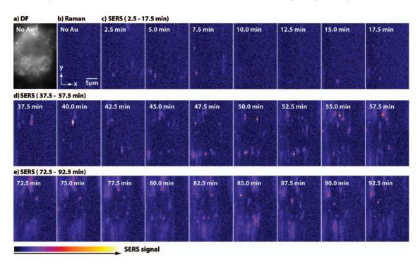
**Fig. 4** Time-lapse SERS image sequences of a macrophage cell with gold nanoparticles. The cell was immersed in Tyrode's solution and gold nanoparticles were added to the solution after taking the images using (a) dark-field and (b) Raman imaging modes. Each image contains  $60(x) \times 200(y)$  pixels. The sample was irradiated with a light intensity of 15 mW/ $\mu$ m<sup>2</sup>.
