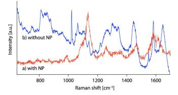
**Fig. 3** Raman spectra obtained from a living macrophage cell (curve a) with and (curve b) without gold nanoparticles (NP). The light exposure for curves (a) and (b) are 10 mW/ $\mu$ m<sup>2</sup> for 1 s and 680 mW/ $\mu$ m<sup>2</sup> for 60 s with 785-nm continuous-wave laser light, respectively.
