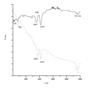
Fig. 1 IR spectra of QDs capped with oleic acid (dashed line) and mercaptoacetic acid (solid line).
