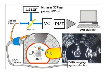
**Fig. 1** A simplified system diagram showing the optical and ultrasound pathways to support the MMC. A cross section of the distal end of the MMC is shown in a phantom artery with a fluorophore target plug placed in the wall. IVUS imaging can clearly orient the SVOF (OF) within the water flushing lumen (F) during the entire positioning procedure.
