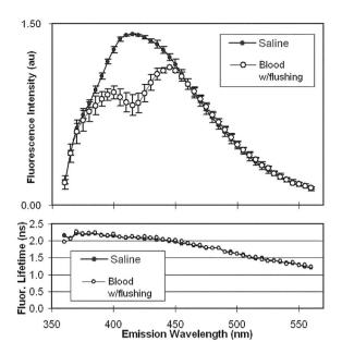
**Fig. 3** Top panel: Comparison of MMC-based fluorescence spectra from an *ex vivo* pig femoral artery for moving whole blood (N=7) conditions against the normalized spectral emission in diluted saline (N=5). Bottom panel: The corresponding fluorescence lifetimes along the emission spectrum.
