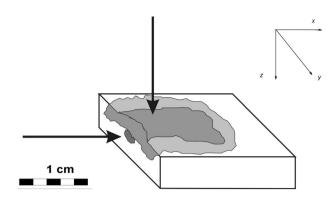
**Fig. 1** Schematic drawing of a paraffin slide from a histopathological preparation of a pigmented lesion. The two arrows indicate the different possibilities for fluorescence excitation; vertical array (z direction): excitation perpendicular to the skin surface, horizontal array (x direction): excitation parallel to the skin surface. The sample holder in the measuring device (LIMES 16-P) allows variation of excitation (scanning) in all three directions x, y, z (see text).
