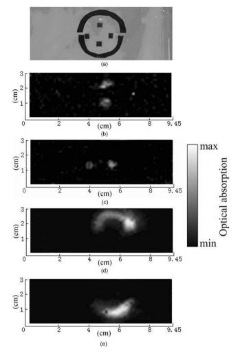
**Fig. 3** Front elevation of (a) the sample, which consists of four different patterns: two lengthways black adhesive tape dots stuck to the front, two transverse black adhesive tape dots stuck to the second layer, a lower half ring of black adhesive tape stuck to the third layer, and an upper half ring of black adhesive tape stuck to the back of three pieces of polymethylmethacrylate. (b–e) are the corresponding reconstructed PA images of the four parts of the sample.
