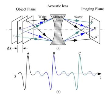
Fig. 1 Diagram of acoustic lens imaging and tomography system.
