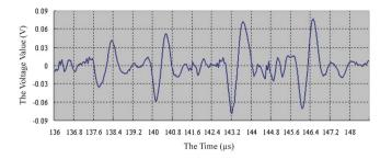
Fig. 4 Reconstructed PA signals from the middle of the four-layer sample.
