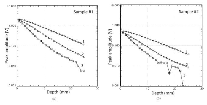
Fig. 5 Amplitude of the acoustic transients as a function of depth for three concentrations of the Intralipid solution (1–0.12, 2–0.24, and 3–0.47%) and two absorption coefficients: (a) 6 and (b) 2 cm<sup>-1</sup> of the subsurface inclusions.
