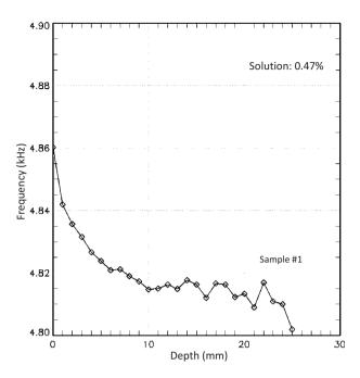
**Fig. 11** Position of the 4.8-kHz peak in the spectrum of the heterodyned signal [see Fig. 10(a)] as a function of depth for sample 1 in Intralipid solution 3 (0.47%).
