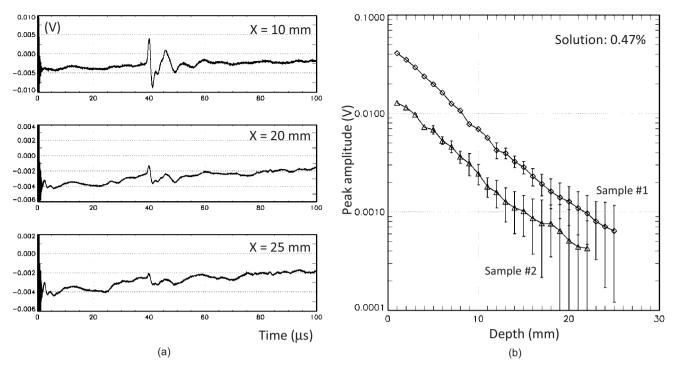
Fig. 6 Time-domain signal and amplitude as a function of depth in Intralipid solution 3 measurements with a low-frequency (0.5-MHz) transducer.
