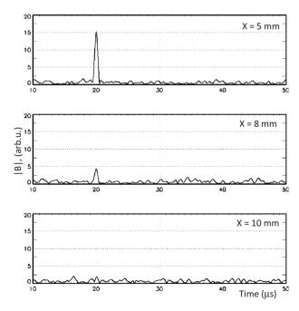
**Fig. 7** Cross-correlation function for sample 1 and chirped optical excitation. Chirp parameters: sweep range, 1–5 MHz; duration, 1 ms. Transducer 3.5 MHz.
