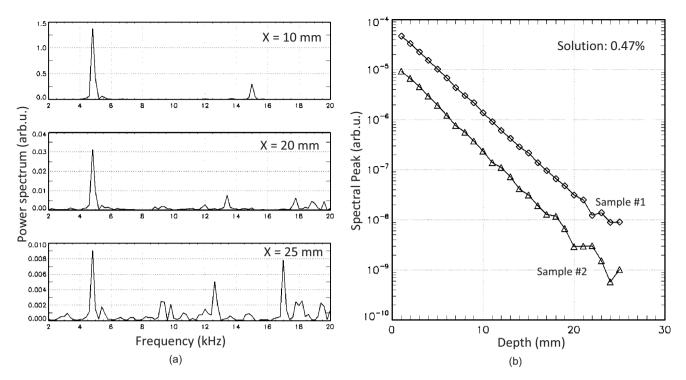
**Fig. 10** Results of spectrum analyzer processing: (a) Power spectrum of the intermediate signal and (b) amplitude of the spectral peak at 4.8 kHz as a function of depth for samples 1 and 2 and Intralipid solution 0.47%.
