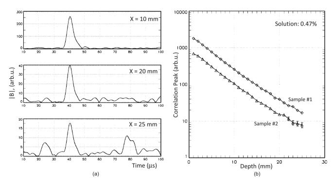
**Fig. 9** (a) Cross-correlation function for sample 1 and chirped optical excitation. Chirp parameters: sweep range 200–800 kHz, duration 5 ms. (b) Magnitude of the cross-correlation peak as a function of depth for samples 1 and 2 in highly scattering Intralipid solution (0.47%). Transducer 0.5 MHz.
