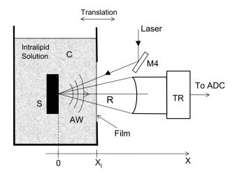
**Fig. 2** Schematic of acoustic wave photogeneration and detection for a test sample immersed in Intalipid solution.
