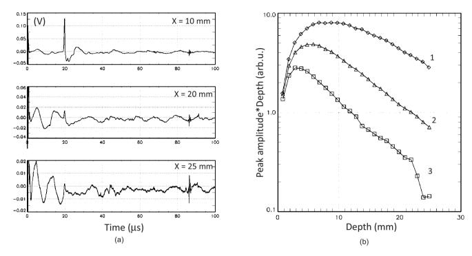
**Fig. 4** Time-domain signal (a) for sample 1 in the high-scattering Intralipid solution (0.47%) at three depth positions X=10, 20, and 25 mm recorded with a high-frequency (3.5 MHz) transducer; (b) product of the signal amplitude and the sample depth versus depth for the three Intralipid solutions (1-0.12, 2-0.24, and 3-0.47%).
