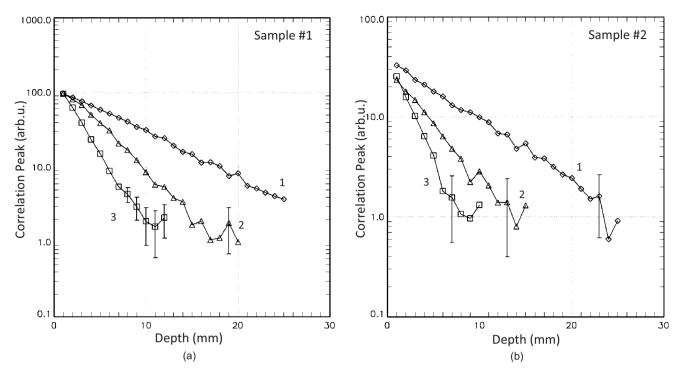
**Fig. 8** Magnitude of the cross-correlation peak as a function of depth for samples 1 and 2 and three concentrations of the Intralipid solution (1–0.12, 2–0.24, and 3–0.47%). Chirp parameters: sweep range 1–5 MHz, duration 1 ms. Transducer 3.5 MHz.
