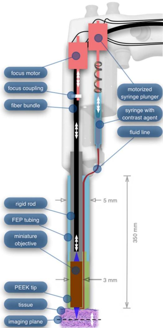
**Fig. 12** Detailed cross-sectional view illustrating the focus mechanism and contrast agent delivery system in the third-generation microlaparoscope. The focus motor couples to the fiber bundle, causing axial movement of the distal end of the fiber relative to the lens. The motorized syringe plunger forces fluid in the syringe to pass through the fluid line, into the tip, and out the tiny orifice at the edge of the system's field of view. (Diagram not to scale.)
