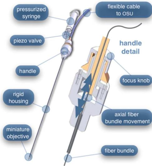
**Fig. 9** The second-generation microlaparoscope. The overall device, shown on the left, incorporated a manual focus mechanism and an integrated dye delivery system that uses a piezo valve and a pressurized syringe. The right side shows a cross-section of the depth/focus knob built into the handle.
