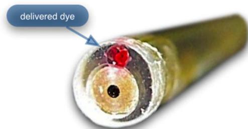
**Fig. 8** Demonstration of contrast agent delivery in the first-generation system. Delivery time was approximately one second to deliver a 1- $\mu\text{L}$  volume.
