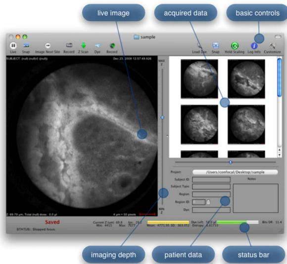
**Fig. 5** Software control system interface. The main window provides the live view and basic controls to run the system. The right side contains previews of data acquired during the procedure along with patient data.
