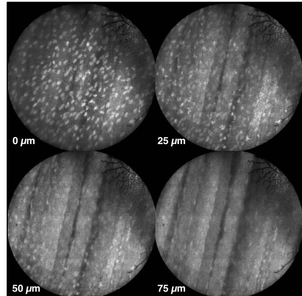
**Fig. 7** Image sequence demonstrating first-generation focus control and the confocal properties of the OSU. Sequence shows the process of incrementally focusing from the epithelial layer (0  $\mu\text{m}$ ) down to the muscle layer of mouse peritoneal wall in 25- $\mu\text{m}$  increments. (Circular field of view is 450  $\mu\text{m}$ .)
