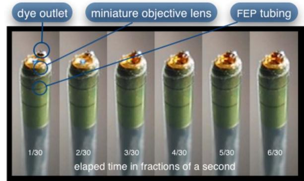
**Fig. 10** Demonstration of the ability of the second-generation microlaparoscope to deliver small volumes of contrast agent to the field of view. In this sequence of images, the operator presses the dye delivery button and the dye is delivered to the distal tip via actuation of the piezo valve. The delivered volume in this example is approximately 1  $\mu\text{L}$ .
