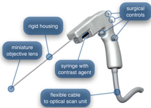
**Fig. 11** The third-generation microlaparoscope. In this view, the rigid steel fiber bundle housing is visible entering into the main handle. A spring-loaded receptacle receives a 1-cm<sup>3</sup> syringe loaded with contrast agents, which couples into the fluid line running to the distal tip. Four buttons allow the surgeon to control focus, contrast agent delivery, and data acquisition. A 6-m-long flexible line connects the microlaparoscope back to the OSU.
