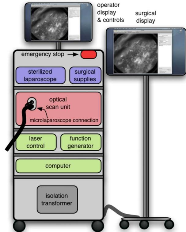
**Fig. 2** Mobile microlaparoscope system. The mobile cart (left) houses the optical scan unit (OSU), surgical supplies, laser source, control systems, computer, and operator controls. The microlaparoscope cable connects to the OSU. The secondary display (right) is placed next to the operative field for live *in vivo* imaging.
