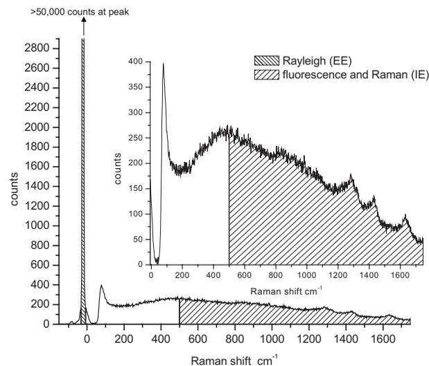
**Fig. 1** Top: Raw typical single 20 ms frame of Andor CCD output with system optimally aligned using 200 mW of 830 nm excitation. Bottom: Sections of emission used to calculate IE ( $\approx 500\text{--}1750\text{ cm}^{-1}$ ) and EE ( $-30\text{ to }+10\text{ cm}^{-1}$ ).
