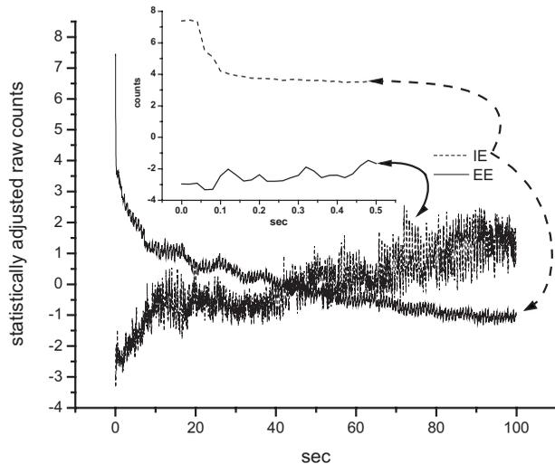
**Fig. 2** Integrated inelastic scattered light + fluorescence and integrated elastic scattered light as a function of time for a single very short and weak mechanical impulse; starting at time  $t=0$  s, followed by active pressure maintenance at 50 g/cm<sup>2</sup>. Inset: same data at shortest times.
