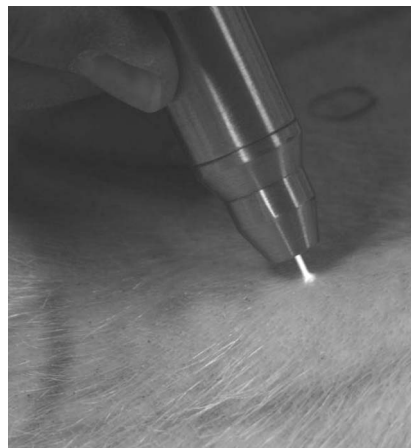
Fig. 1 Photograph of the plasma jet during treatment of tissue (pig ear skin).
