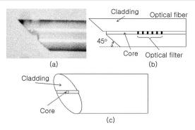
Fig. 1 Processed fiber facet of suggested BOSA, detailed schematic of (b) side view and (c) perspective view.
