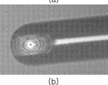
Fig. 3 Infrared camera view of the received modes when both the core and cladding were polished with 45-deg angle. Out-coupling characteristics of (a) out-of-resonance mode and (b) resonance mode of the optical filter.
