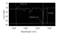
Fig. 2 Transmission spectrum of the optical filter.
