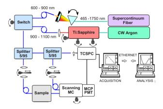
**Fig. 1** Setup of the system for time-resolved transmittance spectroscopy: CW Argon, continuous wave argon laser; MC, monochromator; MCP PMT; microchannel plate photomultiplier tube; TCSPC; PC board for time-correlated single-photon counting.
