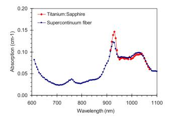
**Fig. 2** Absorption spectra of the breast of a healthy volunteer, as obtained from measurements performed with the two available laser sources. The effect of the laser bandwidth is evident in the estimate of the sharp absorption peak of lipids at 930 nm.
