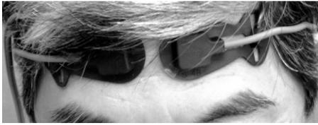
**Fig. 1** Standard probes of a near-infrared oximeter, NIRO-200, attached on the left and right sides of a subject's forehead.
