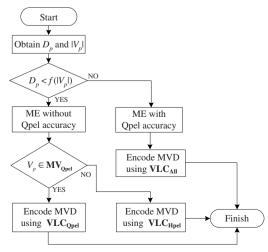
Fig. 2 Flowchart of the proposed algorithm.
