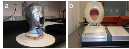
**Fig. 1** Head models: (a) An *ex vivo* tissue head model made with wooden base plates and springs for simulating dynamic movement; the head is made of Styrofoam, clay, and duct tape, which surrounds the whole surface. This can be used for imaging any sample tissue. (b) A commercially available laryngoscopic manikin, for laryngeal examination practice.
