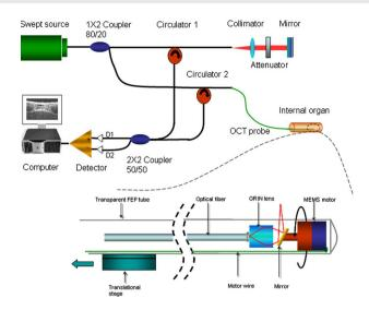
**Fig. 1** Schematic of the swept-source OCT (SSOCT) system and MEMS probe.
