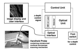
**Fig. 2** Schematic diagram of the confocal endomicroscopy system with a handheld rigid probe used for *in vivo* fluorescence imaging of tumor vasculature in animal models.
