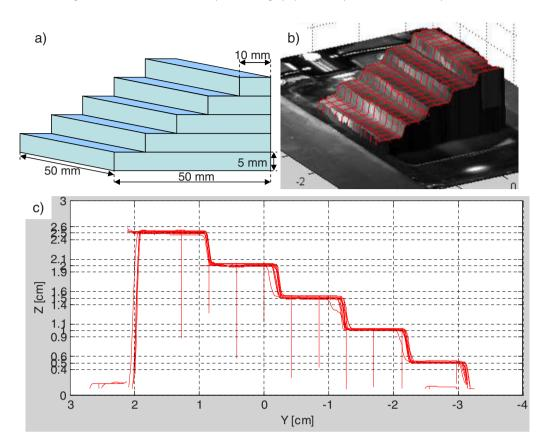
Fig. 3 Staircase phantom used to validate the surface acquisition: (a) schema of the phantom, (b) calculated surface superimposed onto the phantom photograph, and (c) transversal slice of the reconstructed staircase. (Color online only.)
