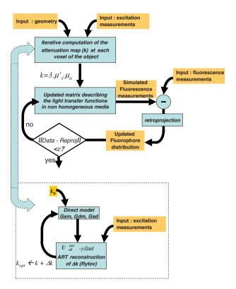
**Fig. 4** Block diagram of the reconstruction algorithm. The reconstruction process is performed in two main steps: attenuation map computation detailed in the bottom dashed box, and iterative fluorescence quantity reconstruction.
