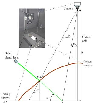
**Fig. 2** Schema of the surface computation within the planar laser acquisition *xz* plane.
