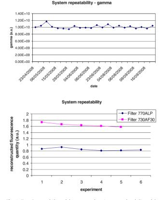
**Fig. 7** Top: Repeatability of the system showing a good stability of the  $\gamma$  parameter over a 5-month period. Bottom: Repeatability of the experiments. The fluorescence quantity is measured in the overall reconstructed volume and is stable with the experiments.
