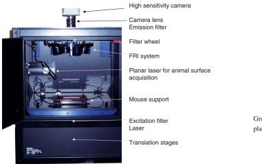
**Fig. 1** Experimental setup. The tomograph is composed of a cooled CCD camera and a laser source coupled to translation stages. The system is also equipped with a filter wheel and an extra planar laser, giving access to the animal surface.
