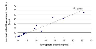
System linearity with fluorophore quantity
