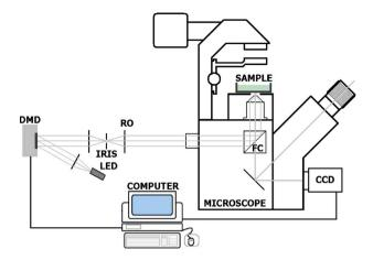
**Fig. 1** Schematic of the spatial-projector setup. The light from an ultraviolet photoactivation light source (LED) was expanded to homogenously illuminate the DMD surface. The UV light pattern was projected through relay optics (RO), the spatial filter (iris), and a DAPI filter cube (FC) onto the flat bottom of a plastic well plate.
