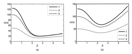
**Fig. 1** Output MSE versus  $\beta$  for two standard test images: (a) Lenna and (b) Baboon, corrupted by additive white Gaussian noise with variances 50 (dotted line) and 100 (dashed line) and by Poisson noise (solid line).
