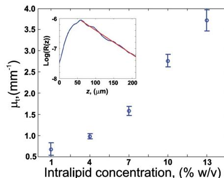
Fig. 2 Attenuation coefficient  $\mu_t$  measured for phantoms with different % w/v concentrations of Intralipid. The inset shows the log-averaged OCT reflectance versus  $z$ , and the linear fit of attenuation (red line) for a phantom with 13% Intralipid. (Color online only.)
