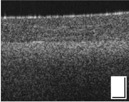
**Fig. 3** Bilayer fibrin phantom, with different Intralipid concentration in both layers. The scale bar represents dimensions  $300 \times 300 \mu\text{m}$ .
