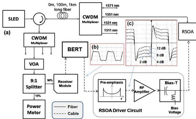
**Fig. 2** (a) Constructed experimental system setup. (b) Waveform of signal from BERT. (c) Waveform with overshoot after pre-emphasis driver. Different levels of pre-emphasis have different output waveforms.
