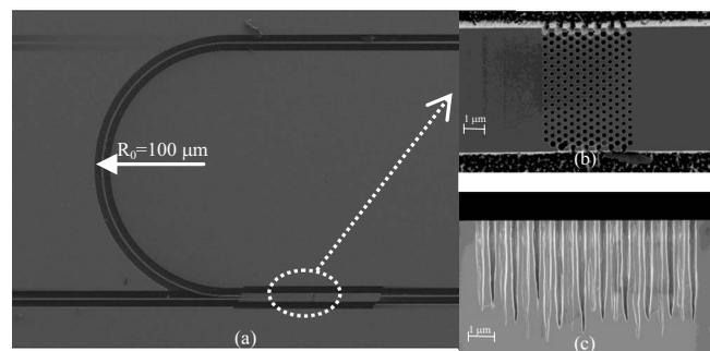
Fig. 3 SEM pictures for the fabricated PBS: (a) top view, (b) internal PhC, and (c) cross section of the etched PhC.
