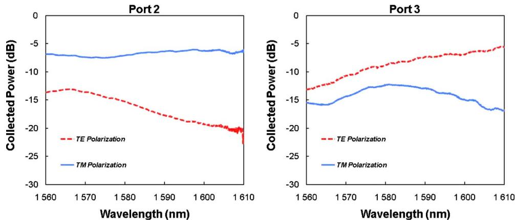
Fig. 4 Measured optical power spectra for the two output ports of the PBS.
