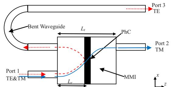
**Fig. 1** Schematic illustration of the PBS with the input and output waveguides.
