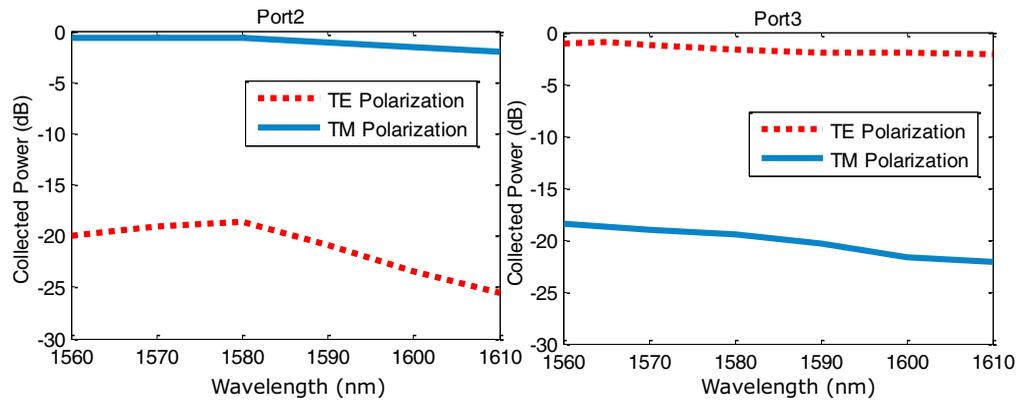
Fig. 2 Optical power spectra at the two output ports of the PBS obtained by 2-D FDTD simulations.
