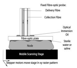
**Fig. 1** Schematic of ESS scanning device (not to scale). The bivalved node is mounted on a mobile scanning stage. It is coupled to a fiber-optic plate above it using a drop of saline or sterile water and gentle but firm pressure. The fiber-optic plate is coupled to a fixed fiber-optic probe with microscope immersion oil. Stepper motors move the scanning stage in an *x*-*y* raster pattern to create a  $20 \times 20$  grid of spectra at 0.5-mm intervals.
