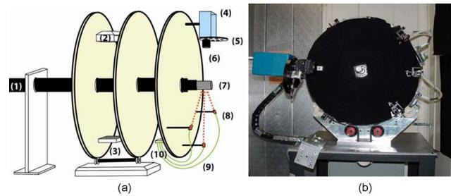
**Fig. 1** (a) Schematic diagram of the FT/DOT/XCT system. The components seen in the schematic diagram are: 1. the sample holder, 2. x-ray source, 3. x-ray detector, 4. CCD camera, 5. filter wheel, 6. lens, 7. phantom, 8. fiber optic collimator, 9. optical fibers, and 10. fiber optic switch. (b) The picture of the system from the front view showing the FT/DOT components.
