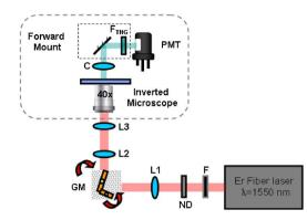
**Fig. 1** Schematic of the experimental setup used for third-harmonic generation (THG). Er Fiber laser is the FemtoFiber FFS laser at 1550 nm; F, RG1000 bandpass filter; ND, neutral density filters; Li, lenses; GM, galvanometric mirrors; C, condenser (NA=1.4);  $F_{THG}$ , bandpass filters (transmittance=512–521 nm); and PMT, photomultiplier tube.
