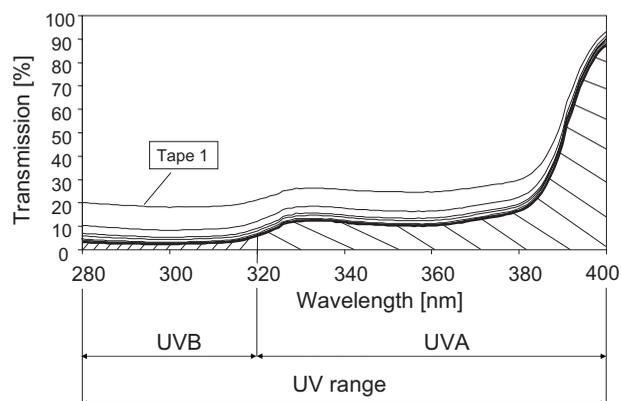
**Fig. 1** Determination of the sum transmission spectrum and the corresponding areas beneath the sum spectrum used to determine the average UVA and UVB sum transmissions (sunscreen sample 7 with SPF 16).
