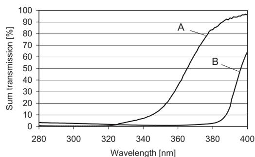
**Fig. 3** Sum transmission spectra of sunscreens belonging to the upper and the lower trend lines in Fig. 2: line A, sample 7, SPF=13; line B, sample 11, SPF=20.
