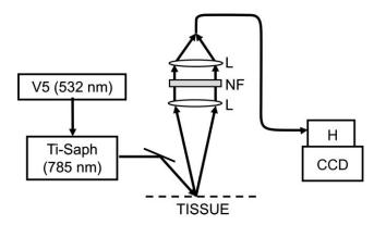
**Fig. 1** Schematic of the Raman system including autofocusing lenses (L), notch filter (NF), axial transmissive imaging spectrograph (H), and liquid nitrogen cooled charge-coupled device (CCD).
