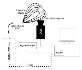
Fig. 1 Setup of the imaging system. MaiTai—Ti:sapphire pulsed laser source, ICCD—time-gated, intensified CCD camera.
