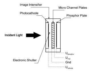
Fig. 3 Scheme of the image intensifier with electronic shutter.
