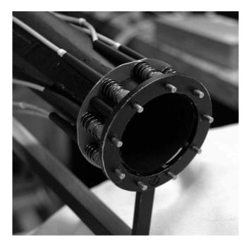
Fig. 2 Emitting fibers located on the ring, spring mounted independently.
