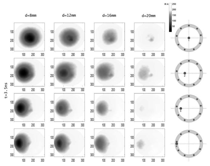
Fig. 8 Images of diffusely reflected light recorded for single time window delayed by 3.5 ns with respect to the maximum of the IRF. The images were obtained for absorbing inclusion located at various depths and different lateral positions.
