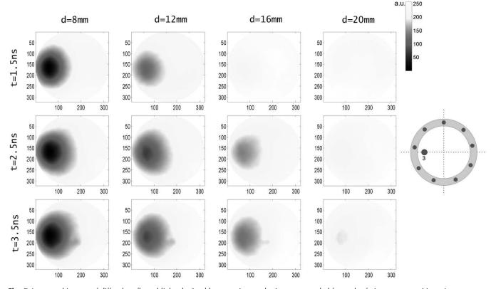
Fig. 7 Integrated images of diffusely reflected light obtained by summing up the images recorded for each of nine source positions. Images were obtained for inclusion located at four different depths end for three different time windows delayed by 1.5, 2.5, and 3.5 ns, respectively, to the maximum of the IRF.
