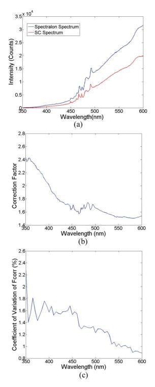
**Fig. 4** Correction for wavelength dependence of the self-calibration channel between 350 and 600 nm (obtained from two scans): (a) raw spectra; (b) correction factor  $F_{\text{corr}}(\lambda)$ ; and (c) coefficient of variation of  $F_{\text{corr}}(\lambda)$  in 10 repeated experiments.
