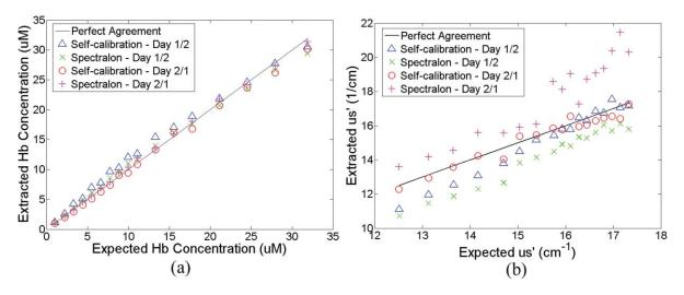
Fig. 8 Extracted versus expected: (a) Hb concentrations and (b) wavelength-averaged reduced scattering coefficients from across-day data analysis, in which phantom 11 from a different day was used as a reference.
