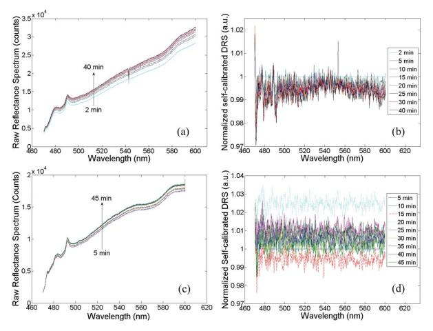
**Fig. 5** Correction for lamp intensity variations: (a) raw spectra from the Spectralon at various time points after the lamp was turned on, and (b) ratio between the Spectralon and self-calibration spectra normalized to the first scan using SC probe B. (c) Raw spectra from the Spectralon at various time points after the lamp was turned on, and (d) ratio between the Spectralon and self-calibration spectra normalized to the first scan using SC probe A.
