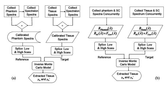
Fig. 2 Data analysis procedures: (a) with Spectralon calibration and (b) with self-calibration.
