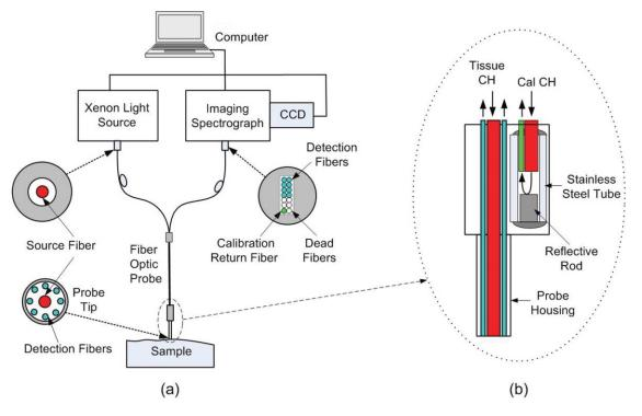
**Fig. 1** Schematic of (a) the UV-VIS DRS system with a splitter-based self-calibration fiber optic probe, and (b) the probe tip showing the termination of the fibers inside the probe housing. The detection fibers and calibration return fibers in the detection bundle are imaged onto the 2-D CCD as two separate tracks. (Color online only.)
