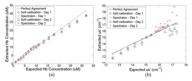
Fig. 7 Extracted versus expected: (a) Hb concentrations and (b) wavelength-averaged reduced scattering coefficients over 450 to 600 nm from within-day data analysis, in which phantom 11 from the same day was used as a reference.
