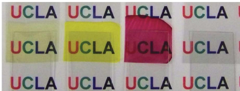
**Fig. 4** Photographs of (from left to right) blue, green, and red PLECs, and two layers of SWNT/PET substrates laminated without any emissive polymer layer.
