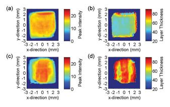
**Fig. 4** Representative terahertz images for an enamel specimen treated with 10 ppm fluoride: (a) baseline AEI reflection intensity, (b) baseline lesion thickness, (c) post-treatment AEI reflection intensity, and (d) post-treatment lesion thickness.
