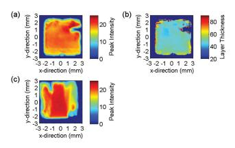
**Fig.** 7 Representative terahertz images for an enamel specimen treated with 2700 ppm fluoride: (a) baseline AEI reflection intensity, (b) baseline lesion thickness, and (c) post-treatment AEI reflection intensity.
