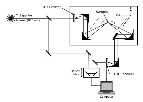
Fig. 1 Schematic of the terahertz-pulsed imaging system in reflection mode.
