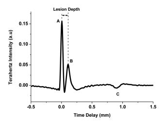
Fig. 2 Terahertz waveform from a single measurement point on a representative demineralized enamel specimen.
