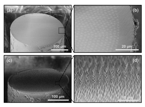
Fig. 1 (a,b) Scanning electron microscopy (SEM) image of the polished imaging fiber end face, from which (c,d) an ordered axicon array was created using a chemical etching method.
