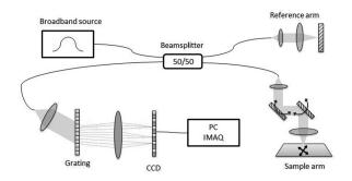
Fig. 1 Schematic of SD-OCT experimental system.
