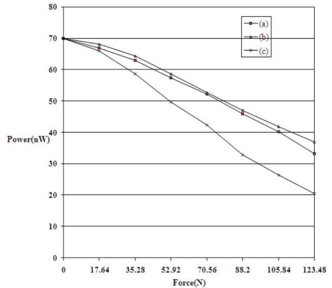
Fig. 2 Optical power detected at optical power meter as a function of the gripping force applied to the steering wheel.
