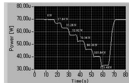
Fig. 3 Optical power variations when varying applied gripping force over time.
